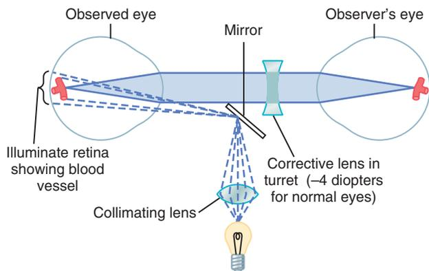
**Figure 50-18.** Optical system of the ophthalmoscope.
