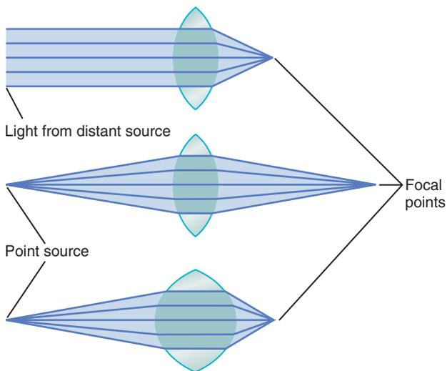
**Figure 50-6.** The two upper lenses of this figure have the same focal length, but the light rays entering the top lens are parallel, whereas those entering the middle lens are diverging; the effect of parallel versus diverging rays on the focal distance is shown. The bottom lens has far more refractive power than either of the other two lenses (i.e., it has a much shorter focal length), demonstrating that the stronger the lens is, the nearer to the lens the point focus is.
