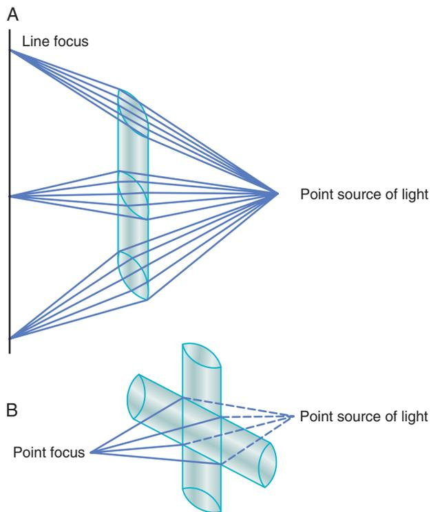
**Figure 50-5.** **A**, Focusing of light from a point source to a line focus by a cylindrical lens. **B**, Two cylindrical convex lenses at right angles to each other, demonstrating that one lens converges light rays in one plane and the other lens converges light rays in the plane at a right angle. The two lenses combined give the same point focus as that obtained with a single spherical convex lens.
